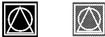
Examples of the same image with and without a screen added to the cliché plate.
